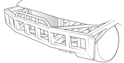
SHS or RHS must not be placed back to back in a horizontal plane. There must be a minimum gap of 30mm before another length of SHS or RHS is placed behind the bumper, for example between the chassis.
